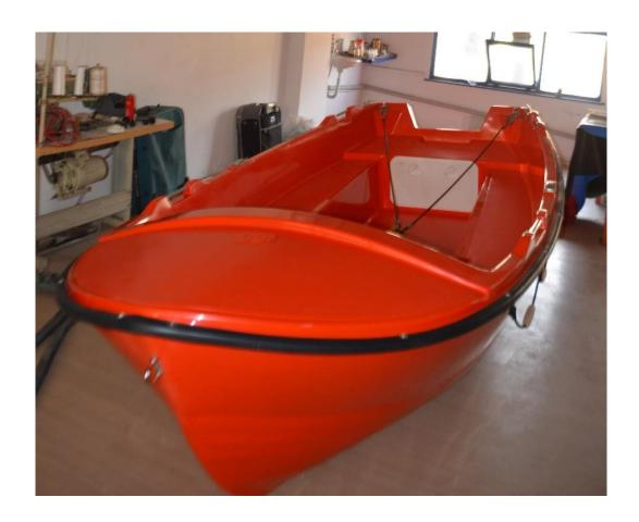
The boat is manufactured of fireproof GRP material. The mold form of the boat is mono-block. Her joints are reinforced with stainless steel bolts as well as lamination which provide waterproof capacity.
